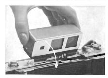
To replace the cover, slide the hinge down over the lock spring until it snaps into place. Swing the cover up; the magnet on top of the camera will hold it in place.
