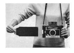
The picture develops outside the camera. While it's developing, hold the tab by the yellow tip, or lay the picture assembly down flat; don't touch or bend the picture assembly or lift off the white paper. Outdoors, don't let the picture assembly flap in the breeze. Develop the picture for the full time recommended in the instruction sheet packed with the film.
