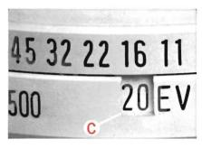
When you turn the aperture control from one EV number to the next higher one you cut the exposure in half. Turn it again to the next higher number and once again you cut exposure in half. And so on, up to the highest EV number — exposure is halved at each step up.
