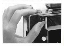
Pull the camera front out as far as it will go, until there is a definite click and the locking bar (A) snaps into place. If the front isn't fully out and locked, your pictures will be blurred.
