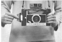
Pull the yellow tab straight out of the camera all the way, swiftly, without hesitating. This starts development of your picture, so begin timing as soon as you get the tab out.
