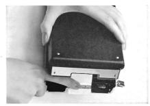
Close the back of the camera, making sure that both sides are locked securely and the white tab is out in the slot.
